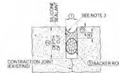
JOINT REHABILITATION DETAILS
